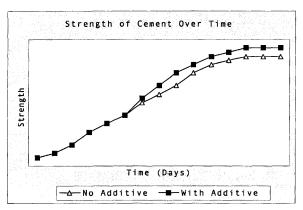
Scenario 5: The additive does not increase the strength of the cement at initial hardening or for some period thereafter, but eventually gives the cement greater strength.
