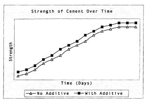
Scenario 4: The additive gives the cement greater strength at initial hardening and at all times subsequent.
