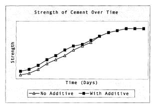
Scenario 6: The additive gives the cement greater strength at initial hardening and for some period thereafter, but eventually a "plain mix" obtains equal strength.
